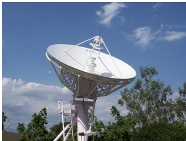
FIGURE 5.2: VSAT ANTENNA AT GEODETIC & RESEARCH BRANCH, DEHRADUN FOR CONTINUOUSLY RECEIVING DATA FROM REMOTE LOCATIONS
